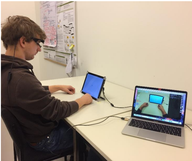
Figure 2: Experimental setup. The subjects interacted only with the tablet. Eye movement data was recorded via tracking glasses.
